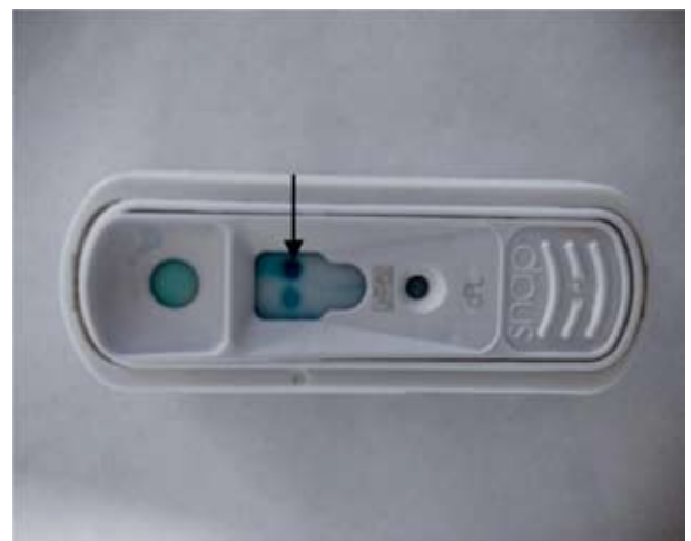
Fig. 1. SNAP cPL test showing intense colour at sample spot (arrow)
