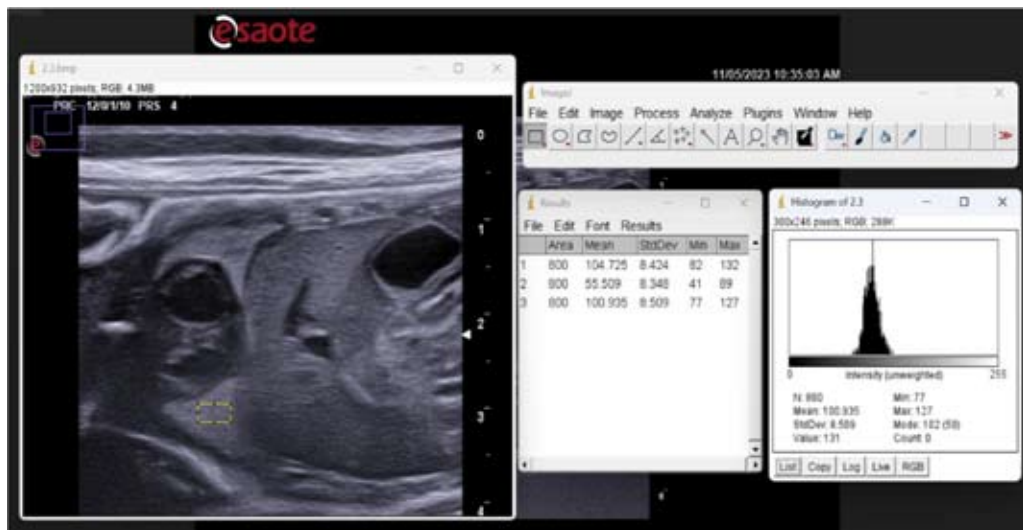
Fig. 2. Analysis of sonographic image measuring the mean grey level, minimum and maximum grey values of foetus with gestational age around 60 days using Image J software.
