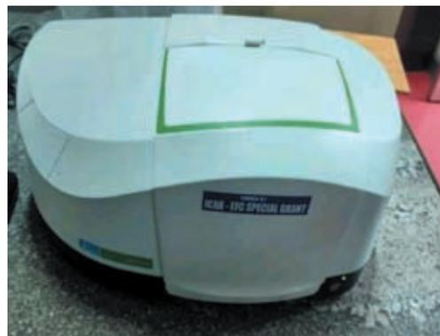
**Fig-4** Perkin Elmer Spectrum 2 Infra-red Spectrophotometer- USA
