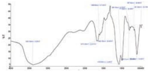
**Figure 5:** Infrared spectrum from goat A<sub>1</sub> showing struvite bands at 3401, 1440, 1670 and 995.16 cm<sup>-1</sup>
