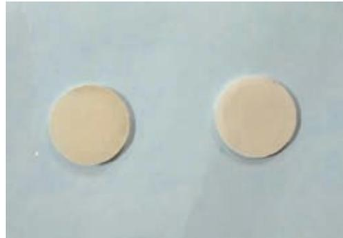
**Fig-3** Prepared pellets of KBr and urolith for FTIR – ATR spectroscopy
