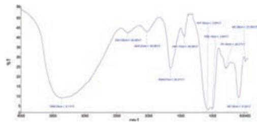
**Figure 8:** Infrared spectrum of goat A<sub>4</sub> showing struvite bands at 3360, 1441, 2321, 1654 and 1000.14 cm<sup>-1</sup>
